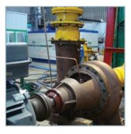
Test Bed at Pumpsense is fully compliant with the requirements of ISO 9906. Test set up is completely automated for flow control and data acquisition.
