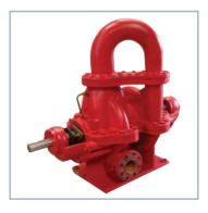
Two stage NFPA20 Split Case fire pumps incorporate two double entry impellers for high suction lift capability and complete axial thrust balance. The pumps are available for rated flows up to 1500 gpm and heads up to 300 m at 2950rpm.
