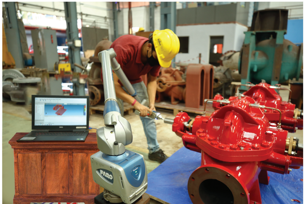
High accuracy dimensional measurement using Faro Arm to check conformance with existing installation
