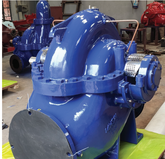
Original: Flowmore Model 5822-400x350 Replacement: Pumpsense model 14HS21 for Tata Steel
