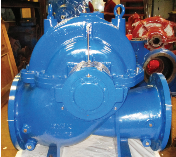
Original: KSB Omega 350-430B Replacement: Pumpsense model 16HS19 for an Australian Customer
