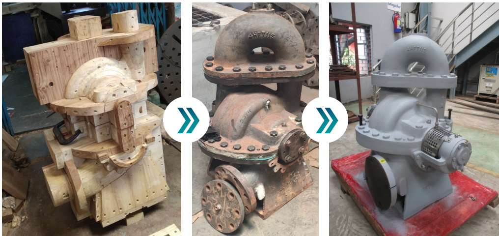
Original: Weir Model Duoglide DQA 100/125 Replacement: Pumpsense model 4HFT11S for an UK based Customer
